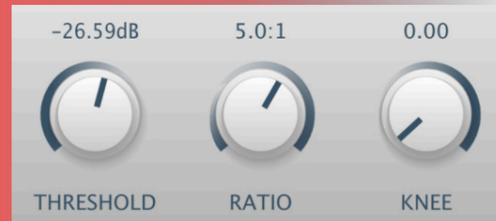
The compressor uses a program-dependent attack and release influenced by old hardware making the compression sound characterful and dynamic. The RMS detection means that Schlap detects the average loudness of a signal, resulting in sudden short peaks being uncompressed so that they can attack hard and sound heavy hitting.
